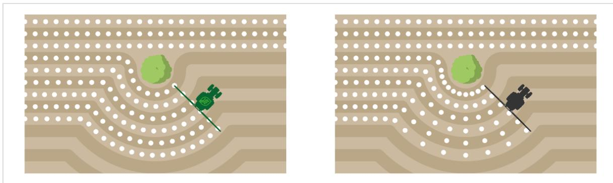
*WEED-IT PWM technology that can compensate for the driving speed (left image) and other PWM technology (right image) that can't and resulting in outer boom parts applying too less spray liquid.*
